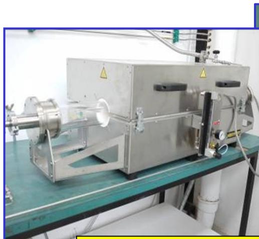
Static corrosion tests
