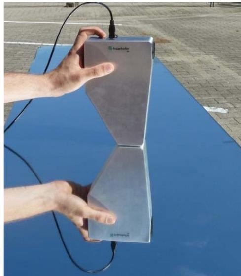
Mobile spectral reflectance measurement
