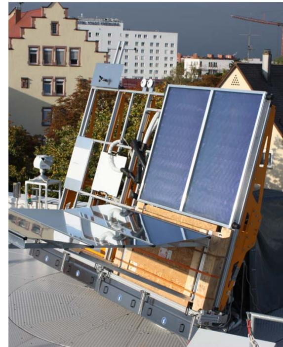
Prototype of RefleC-Collector
