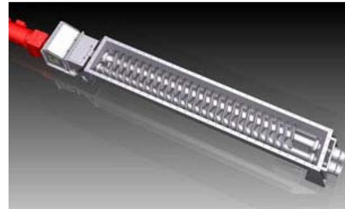
Screw heat exchanger used with phase change materials for latent heat storage
