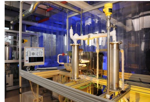
Test bench for salt hydrates
