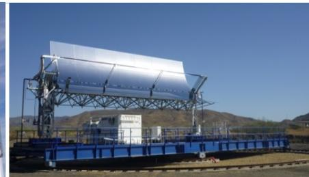
Rotary test bench for parabolic trough collectors (KONTAS)
