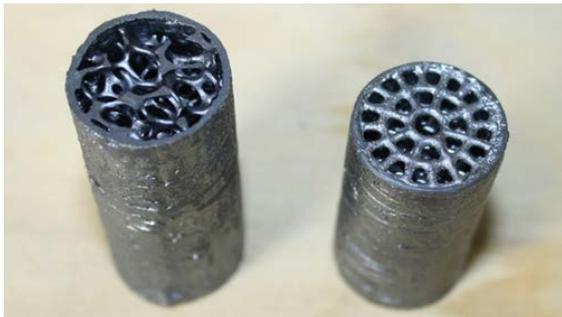
Engineered cellular SiC tubes from SUPSI and Yeungnam University tested for solar gas turbine application
