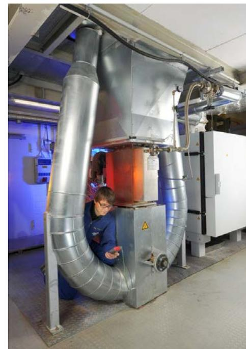
Test facility for particle based heat exchanger for steam generation
