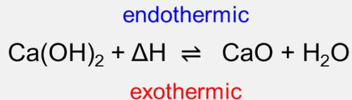
Gas-solid reaction for thermochemical energy storage between 400 and 600 °C
