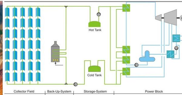
Molten salt plant schematic
