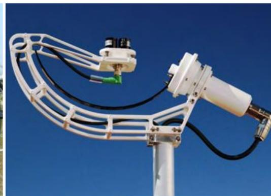
Twin Rotating Shadowband Irradiometer
