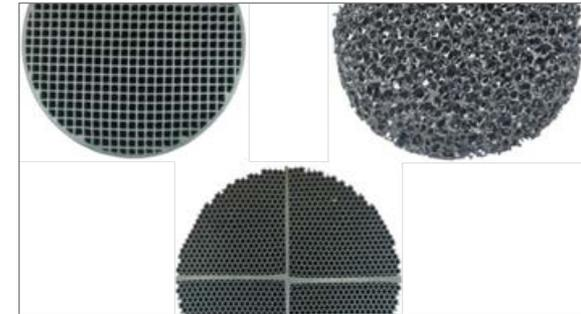
Volumetric absorber structures
