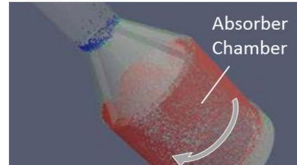
Centrifugal particle receiver (CentRec)
