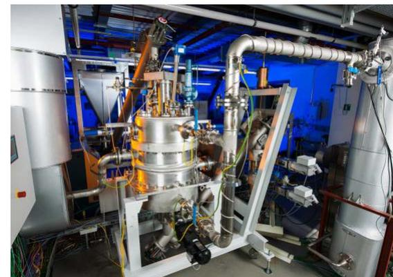
100 kWh moving bed test setup
