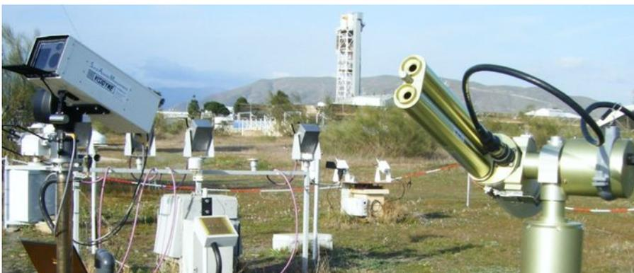
Equipment for sunshape measurement: Visidyne's SAM (left) and CIMEL sunphotometer (right) at the Plataforma Solar de Almería
