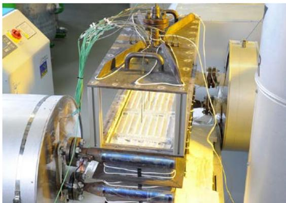
10 kWh plate heat exchanger test setup
