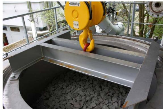
Inner chamber of testbed with storage material
