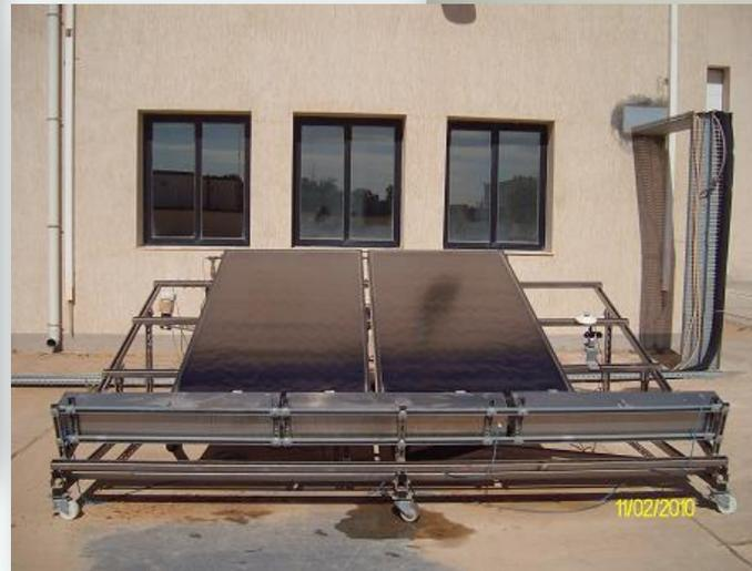
**Solar Water heating Systems Test Facility**
