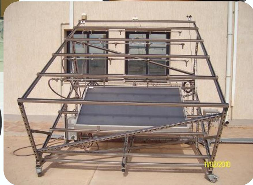
← Collector rain penetration Test
