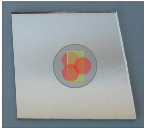
Figure 1: Illustration of the positioning of the measurement spots on a reflector sample. The grey circle represents the minimum area of the erosion experiment (2.5 cm diameter), the red circles stand for the D&S measurement spots (1 cm diameter with allowed overlap) and the green rectangle for the measurement spot of a Lambda 1050 spectrophotometer from Perkin Elmer (17 x 9 mm 2 ) in the 0° measurement position. This spot shall be rotated two times by 90°.
