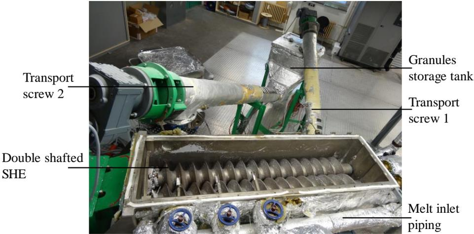
**Figure 2. Experimental setup of the active latent heat storage with a screw heat exchanger (SHE): in the picture, the SHE and the PCM-circuit are shown [4]**
