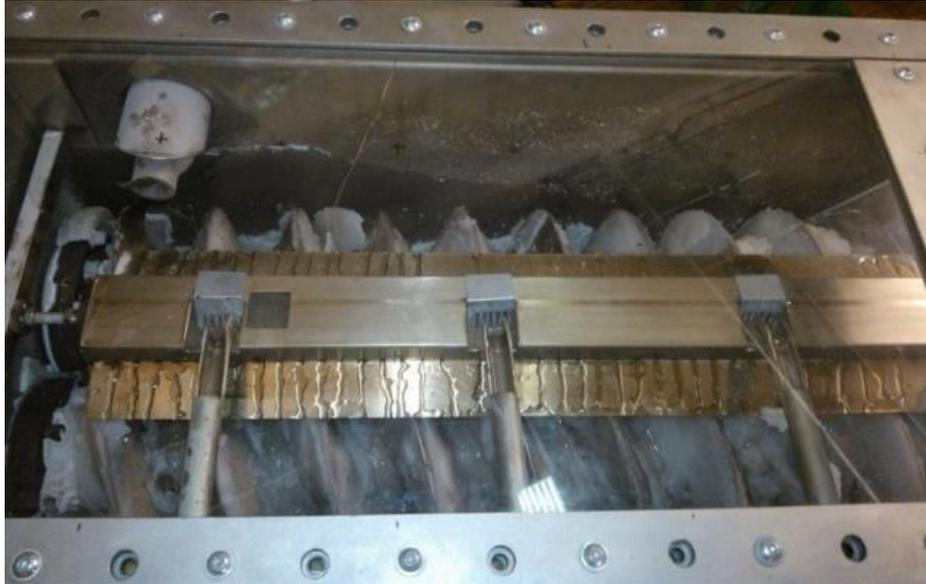
*Figure 6. Inlet system for liquid PCM into the SHE*
