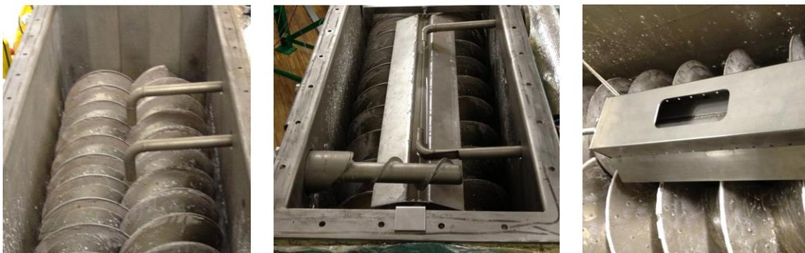
*Figure 5. Different salt distribution systems in the prototype. Left: original system from supplier, middle: first improved prototype; right: optimized system*
